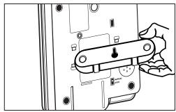
Figure 6 - Phone Base for Wall Mounting
